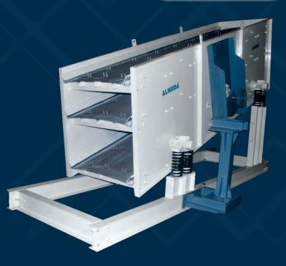
The bolted and welded steel structure forms the screen frame that accommodates the screen mesh and drive unit. The screen comprises of an eccentric shaft, made out of alloy steel and two no. of heavy duty double spherical bearings with dust and watertight seals, for efficient operation and low maintenance.
